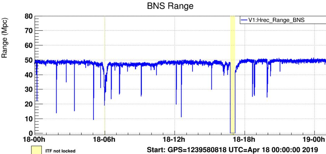
High duty cycle (more than 90%) with a sensitivity of  $\sim 50$  Mpc BNS range (almost x2 higher than O<sub>2</sub>)
