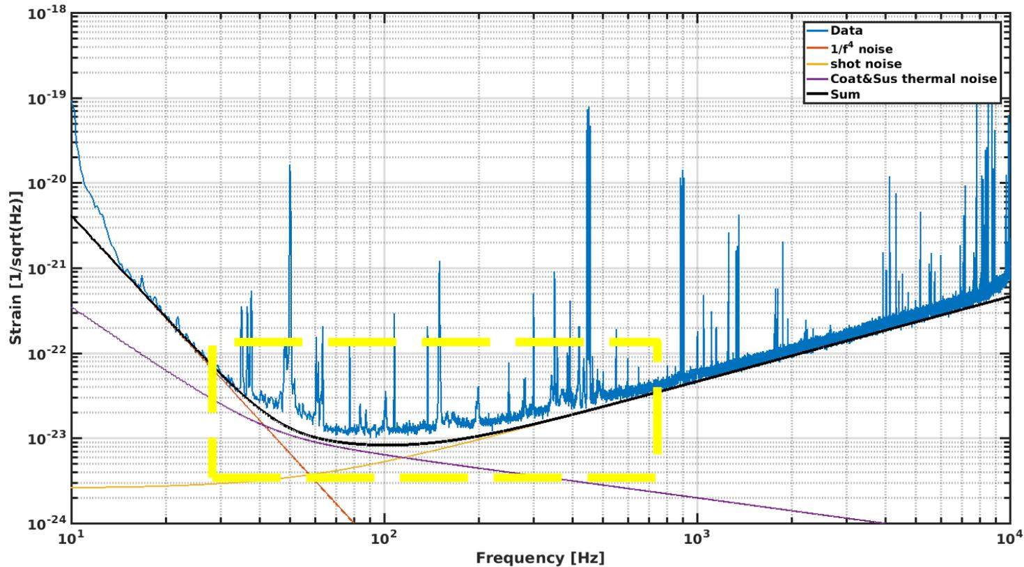
The noise budget accounts for all the known technical noises, but cannot account for the noise “in the bucket”, in the region between 40Hz and 400Hz. This is what we call the “flat” noise
