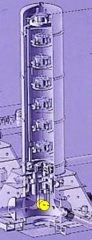
Reduces mirrors seismic vibrations
