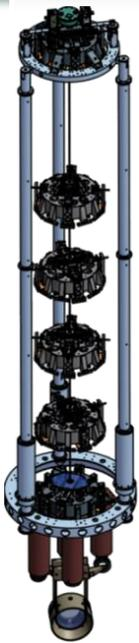
▶ Seismic isolation: **superattenuators** (same as in iVirgo)
