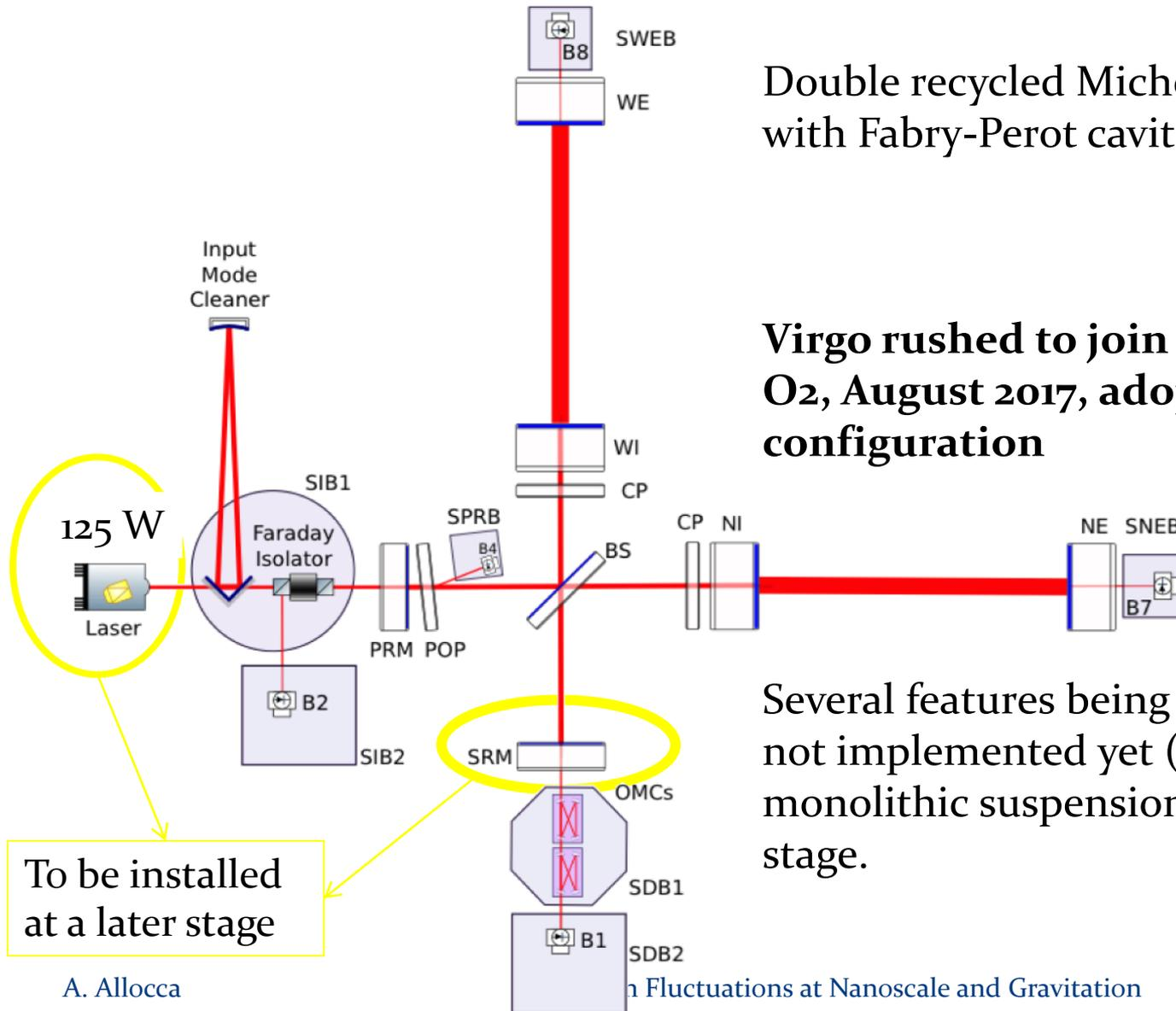
Double recycled Michelson interferometer with Fabry-Perot cavities in each arm.
