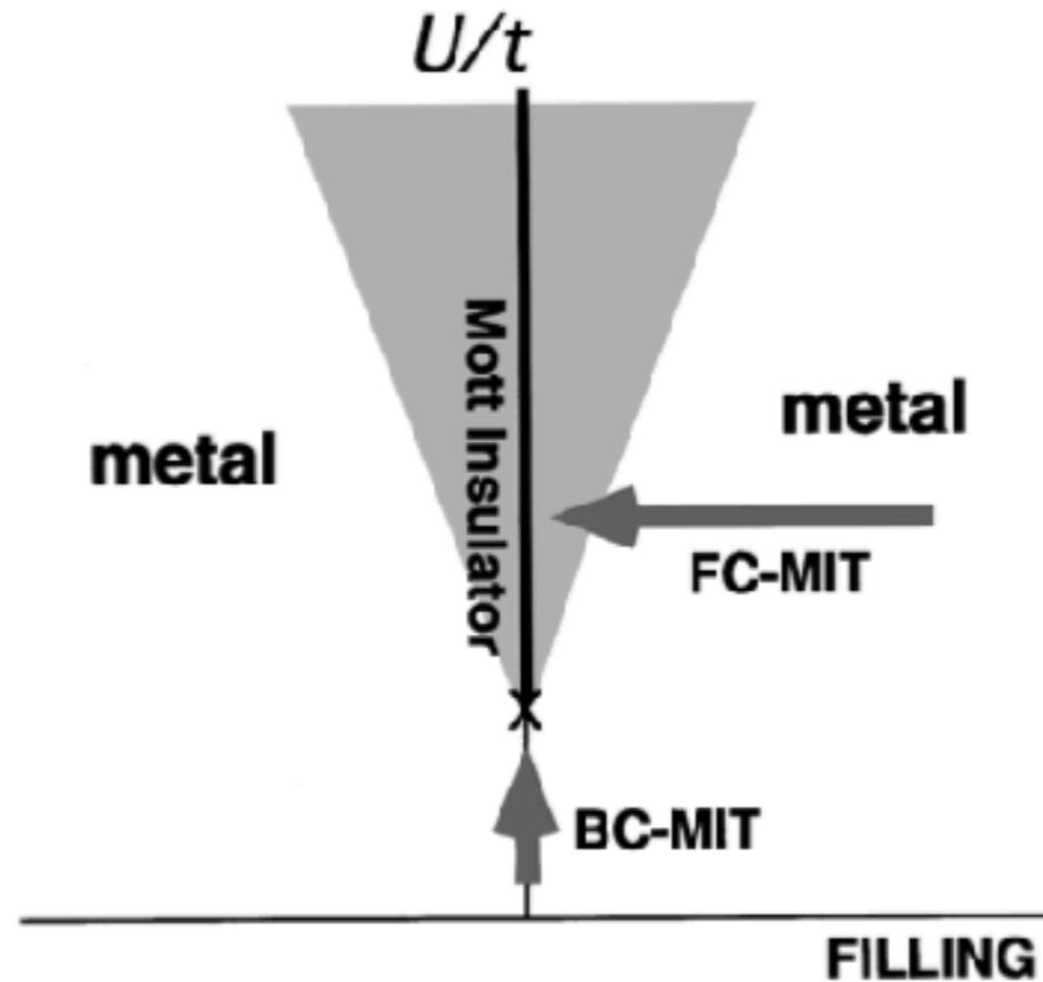
FIG. 1. Metal-insulator phase diagram based on the Hubbard model in the plane of  $U/t$  and filling  $n$ . The shaded area is in principle metallic but under the strong influence of the metal-insulator transition, in which carriers are easily localized by extrinsic forces such as randomness and electron-lattice coupling. Two routes for the MIT (metal-insulator transition) are shown: the FC-MIT (filling-control MIT) and the BC-MIT (bandwidth-control MIT).
