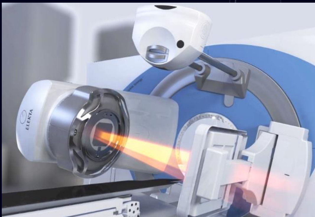
Dynamic multileaf collimator to shape the beam (up to 160 individual leaves)
