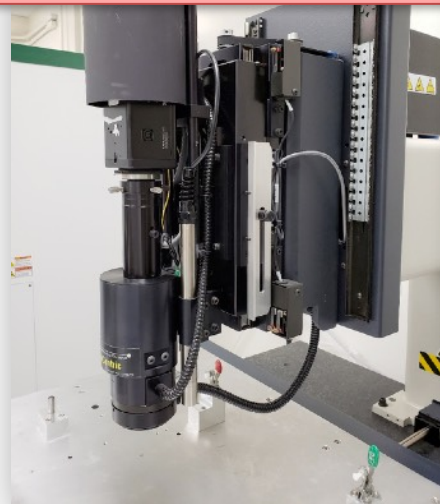
Pull Tester Test strength of wire bonds
