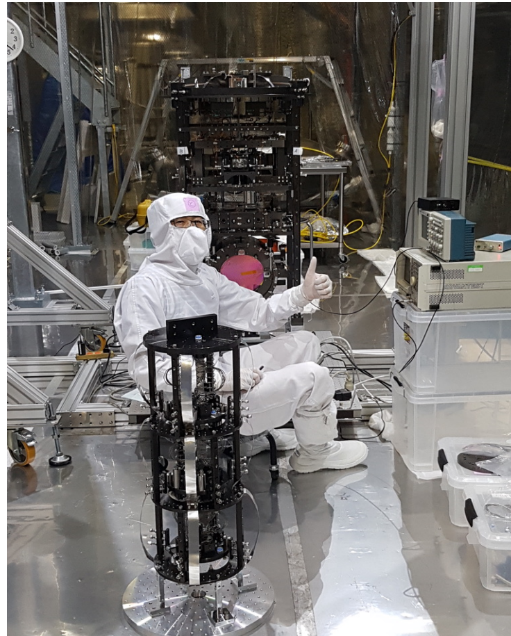
Assembly of the final attenuator at the KAGRA site
