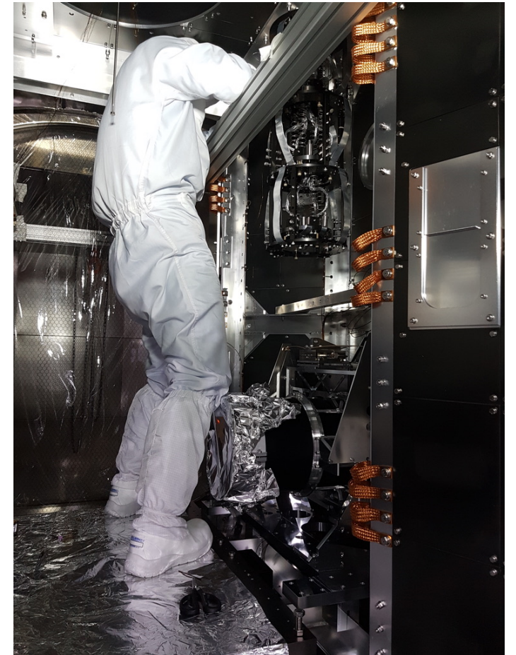
Heat link attenuator integration into the cryostat
