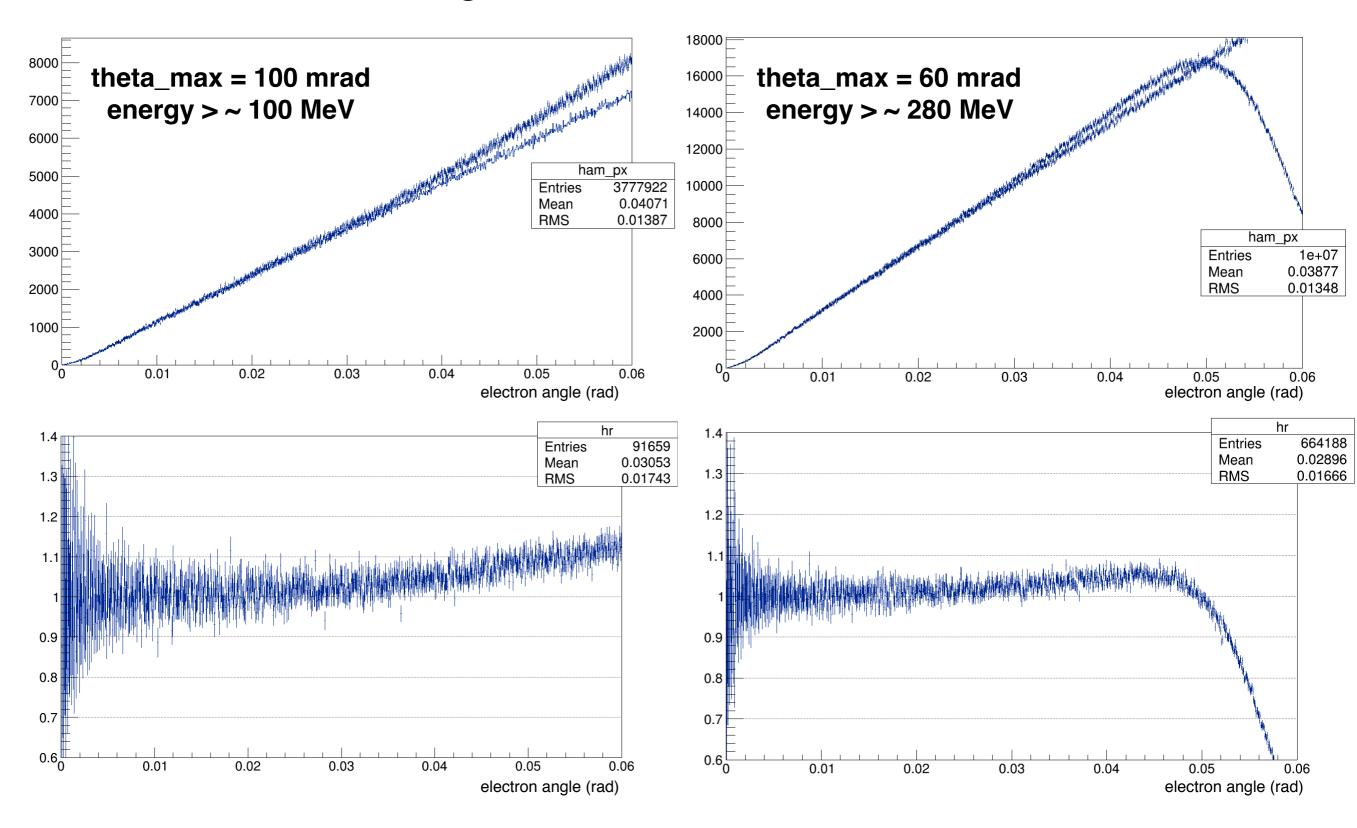
• **Question**: how to preserve the high angle region, but do not waste computing time? Max angle cut in generation distorts the spectrum.
