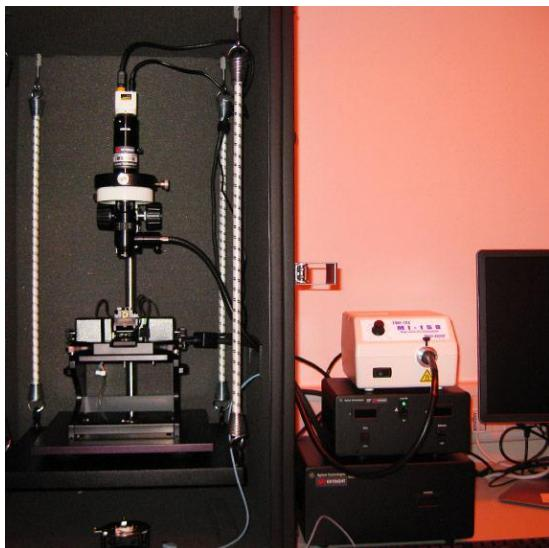
Both STM and AFM scanners can be used with the sample placed inside a protective atmosphere (Ar) at a defined temperature
