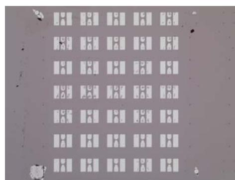
Graphene-based RF devices on HR Silicon
