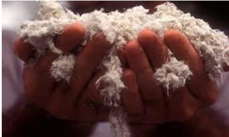
iron contamination  $[(\text{Mg},\text{Fe})_3(\text{Si}_2\text{O}_5)(\text{OH})_4]$  imparts radical reactivity, hence toxicity, to any chrysotile outcrop
