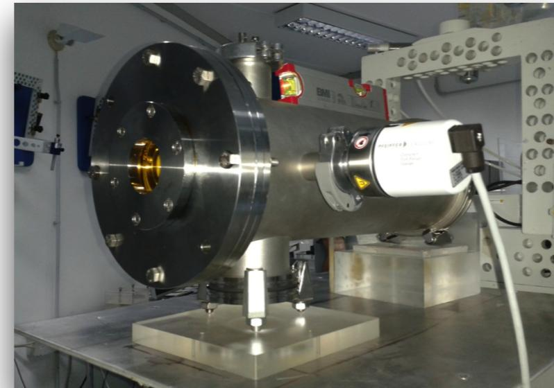
Faraday cup based detector for the absolute determination of the released dose
