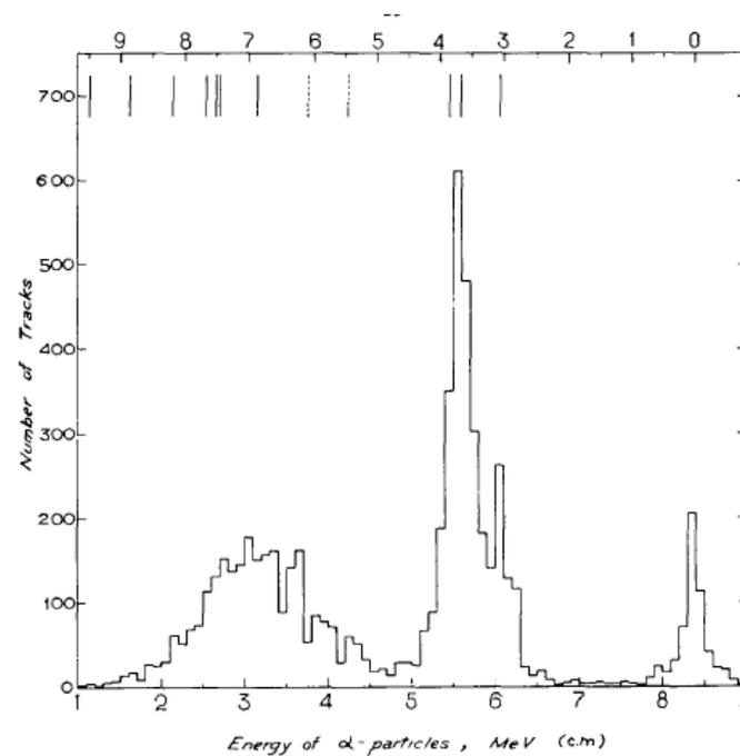
Fig 1. Alpha-particle spectrum from the  $^{16}\text{O}(n,\alpha)^{13}\text{C}$  reaction at 14.1 MeV.
