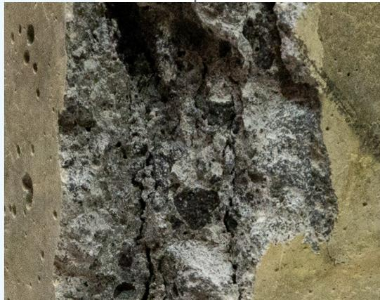
Being a composed material, **CONCRETE** breaks very slowly when increasing the compression, with **fractures** propagating along **preferential lines** surrounding the aggregates. This phenomenon could be responsible of the long-range correlations quantified by **increasing** values of  $q$ .
