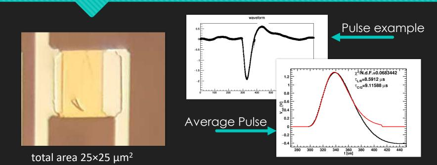
Pulse detected on laser trigger Average photons per pulse << 1
