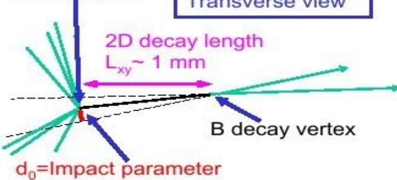
**Lepton ( $e, \mu$ ) + displaced track trigger**
