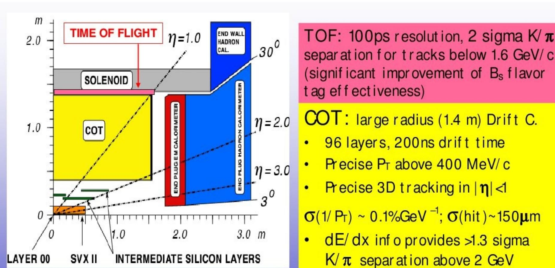
TOF: 100ps resolution, 2 sigma  $K/\pi$  separation for tracks below 1.6 GeV/c (significant improvement of  $B_s$  flavor tag effectiveness)
