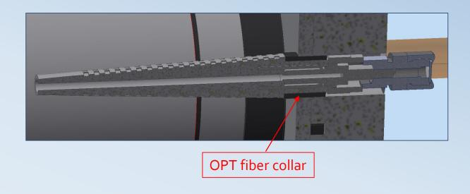
The SMA connector is sealed with a tango black gasket with 2 mm thickness.
