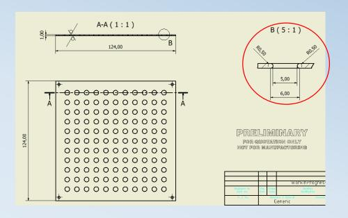
Cathode made by conductive copper foil with holes to ensure gas inlet.
