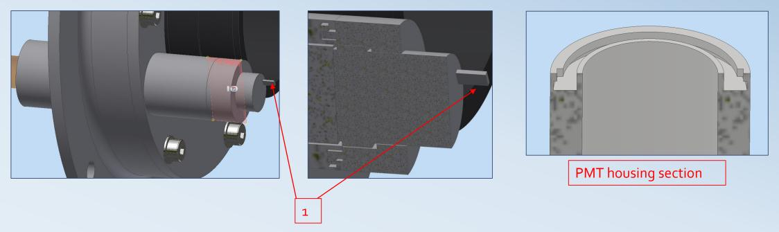
The connection housing – socket is made by two teeth to achieve the light-tightness.
