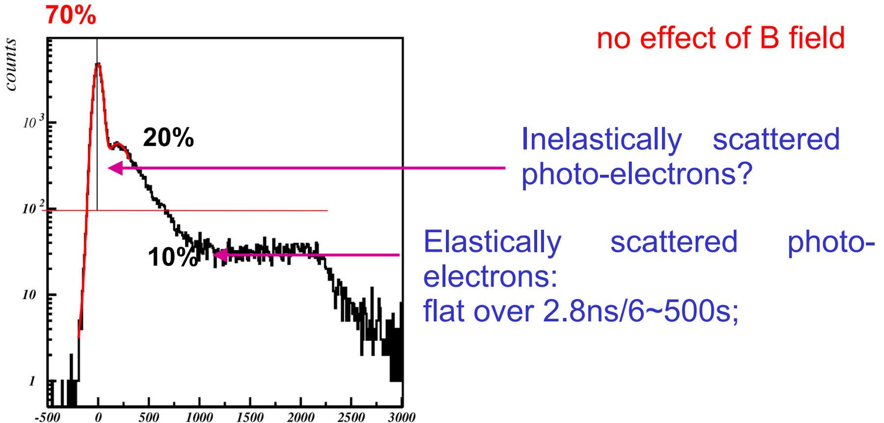
$\rightarrow$  rms of the TDC distribution  $450\text{ps} \rightarrow \sim 80\text{ps}$ , for N photons again use only the 'first' ones
