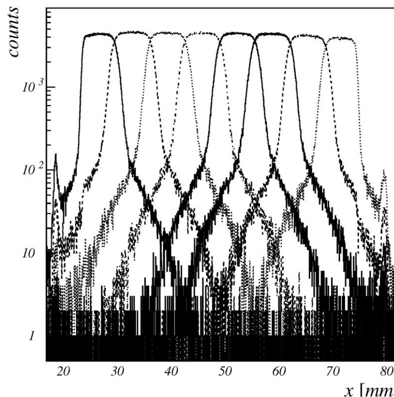
Response similar to 2x2 MCP PMT: charge sharing and long tails due to photo-electron back-scattering.
