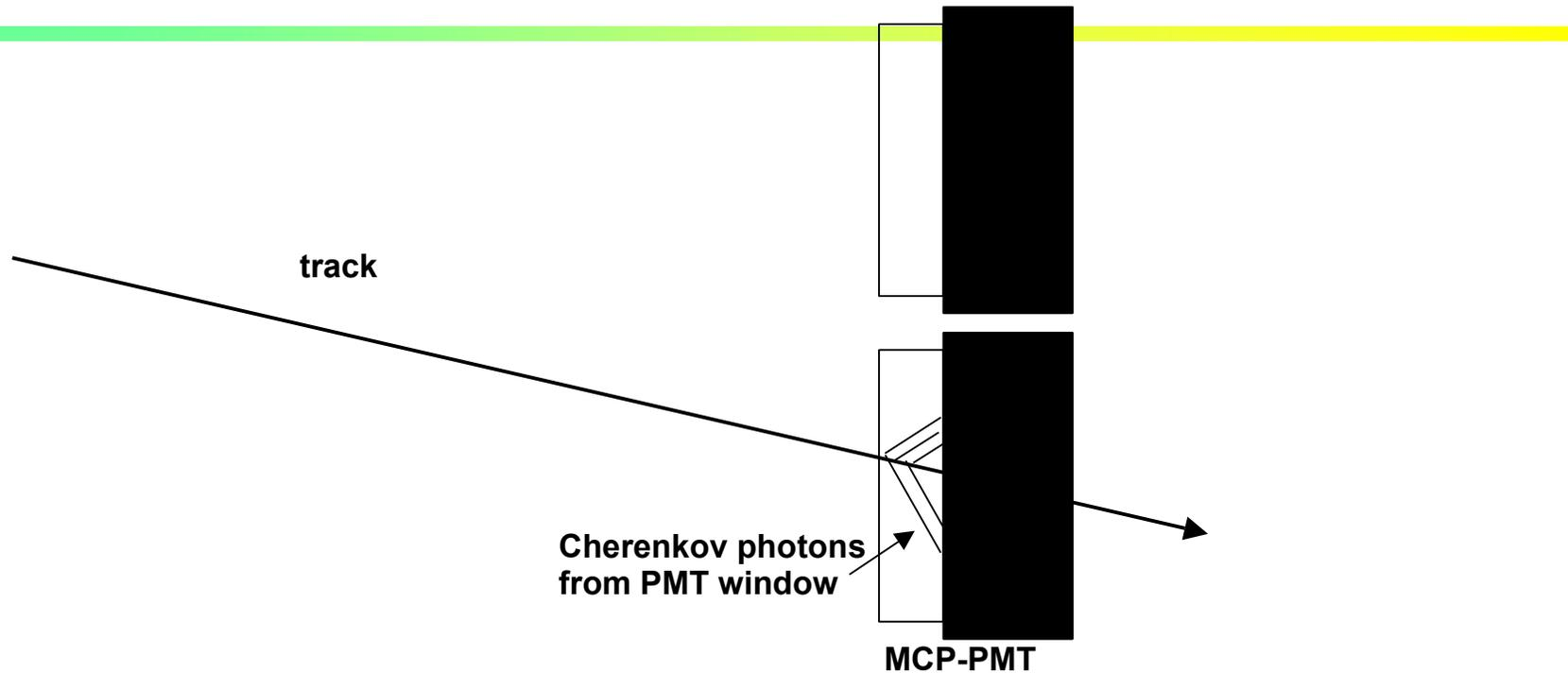
Typical situation in TOF measurements; not the same as multiphoton hits on a single pad.
