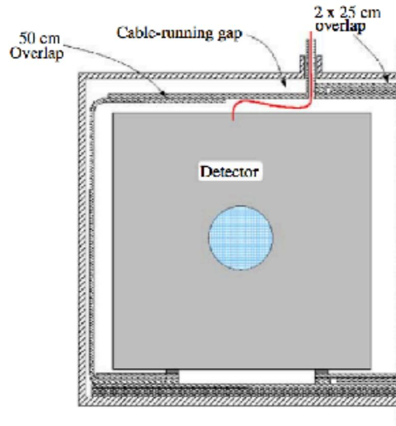
**1 cm acrylic HHV shield configuration as from DRIFT**
