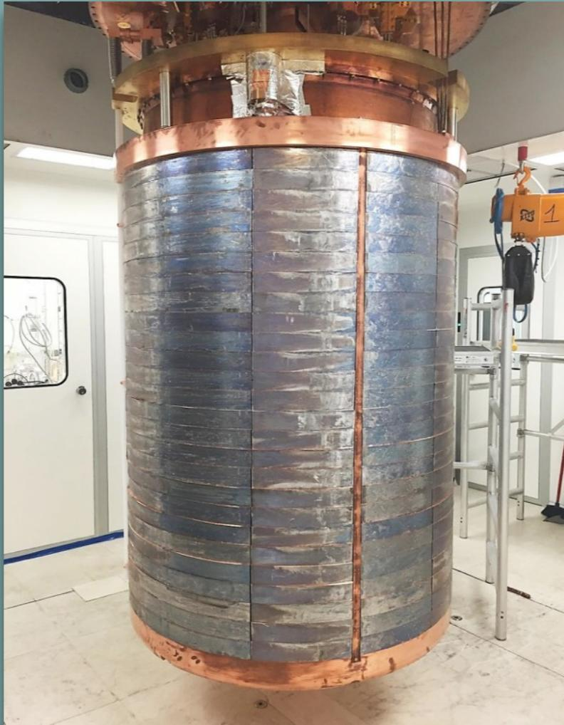
**Lateral and bottom shielding with 6cm - thick  $^{210}\text{Pb}$  - depleted roman lead**
