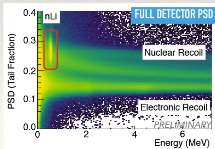
Powerful combination of PSD in the prompt and the delayed signal
