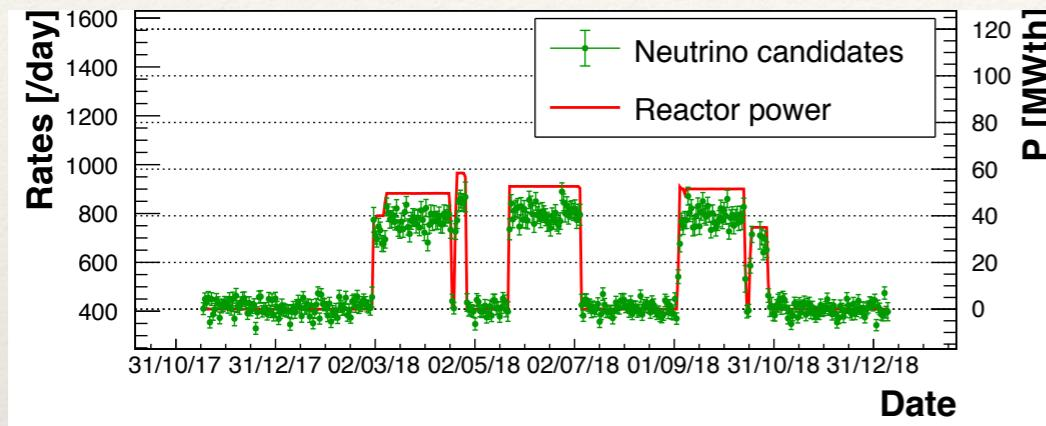
Accidental background due to the reactor activity mitigated by the large detector shielding
