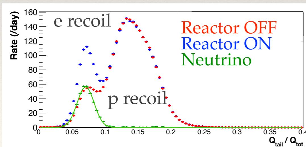
The dominant background is induced by cosmic-rays. The main contribution is a p-recoil in the prompt signal, followed by a n-capture coming from the same cosmic shower efficiently rejected by the Pulse Shape discrimination PSD
