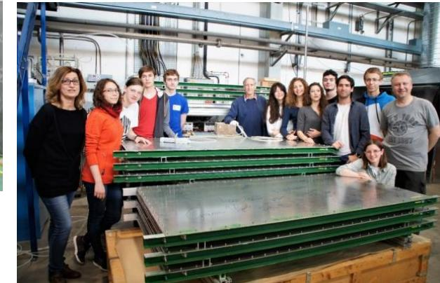
3 MRPC planes with 24 strips each read at both ends  $\rightarrow$  144 readout channels
