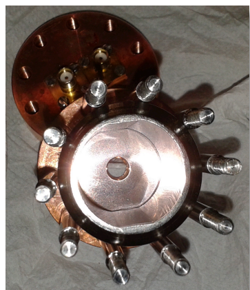
Bulk Nb cavity ( H_{c2} 0.6 T)
