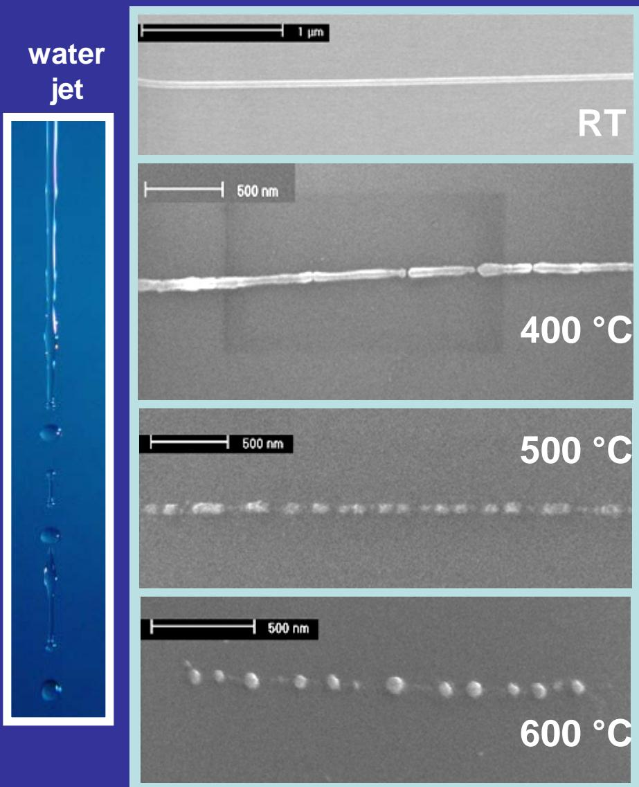
30-nm Cu wire on  $\text{SiO}_2$  substrate
