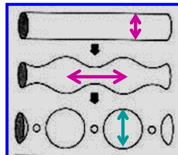
$$\begin{aligned} & 2r \quad \downarrow \\ & \lambda \quad \text{surface diffusion} \\ & d \quad \downarrow \\ & d_s = 3.78 r \end{aligned}$$
