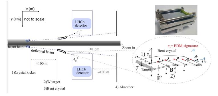
Need to study a beam extraction scheme for the LHC (in collaboration with CERN)
