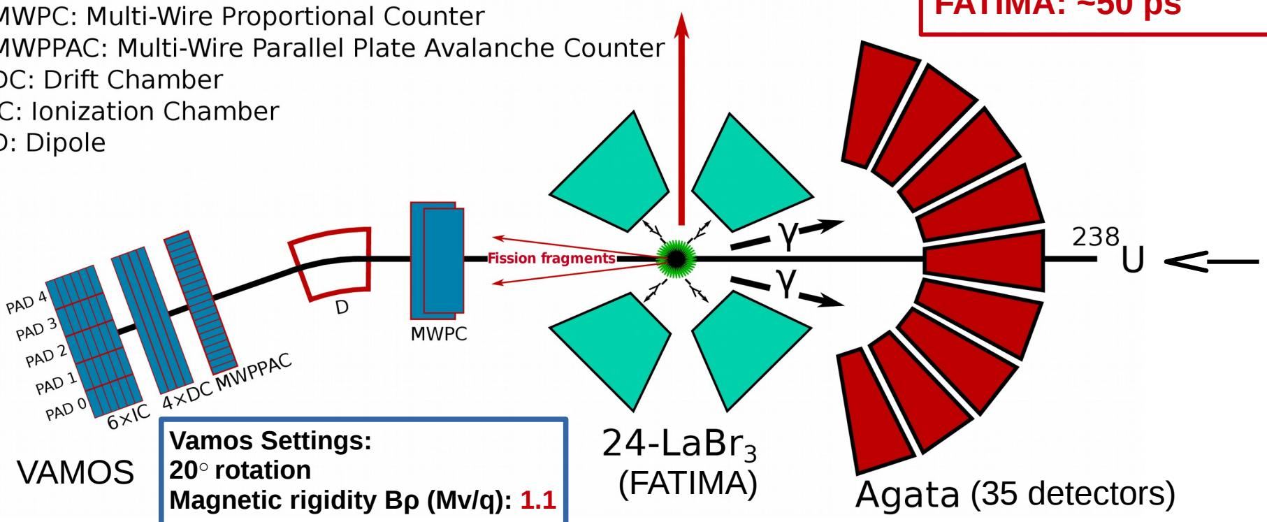
**AGATA** is an array composed of high-purity segmented germanium detectors.
