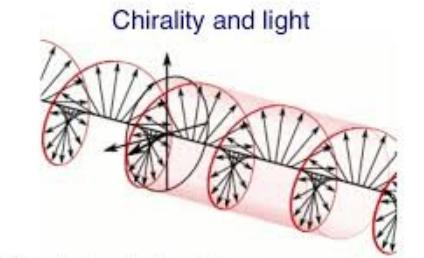
Circularly polarized electromagnetic wave
