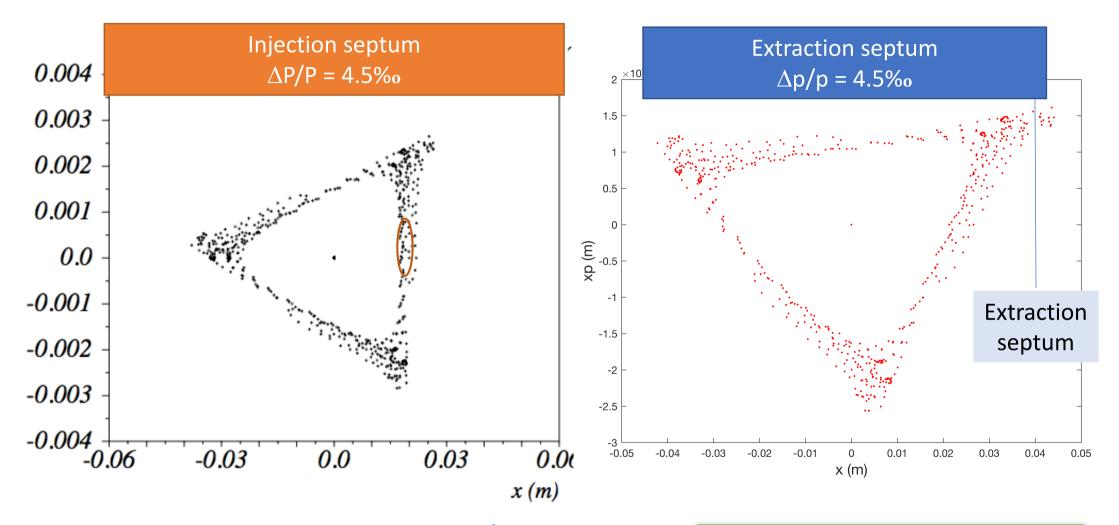
Mad8 tracking with initial energy  $\Delta P/P = -0.0045$ , average radiation energy loss (no fluctuations), RF off, collimators included
