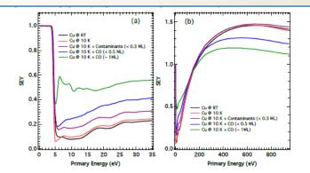
WP1-Fig. 2: a) LE-SEY and b) SEY curves measured at 10 K on a polycristalline Cu sample clean (red) and in the presence of 0.3 ML of adsorbed residual gases (purple) and of 0.5 ML (blue) and 1 ML (green) of adsorbed CO. The LE-SEY and SEY curves measured on the clean sample at RT are shown for comparison (black). [Pub. WP-1:1]
