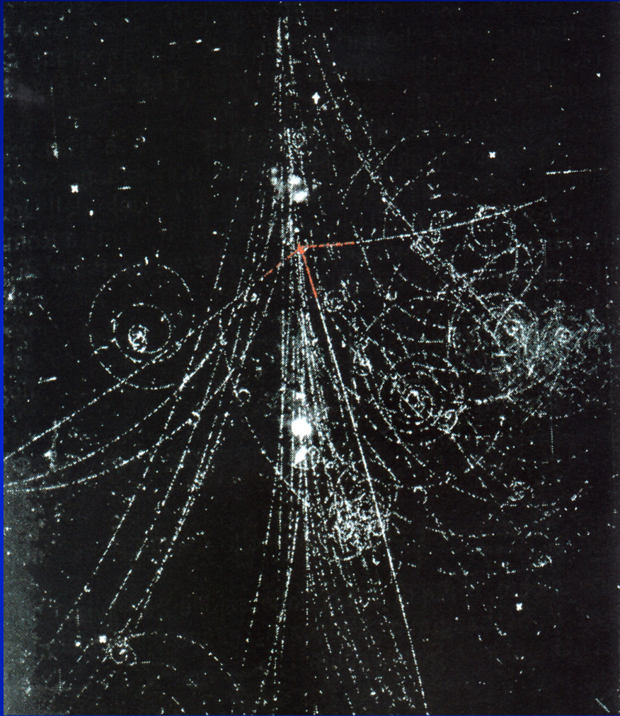
frame of the bubble chamber: in red the point at which the photon, interacting with a proton, has created a pair of pions; the third trace is that of the proton
