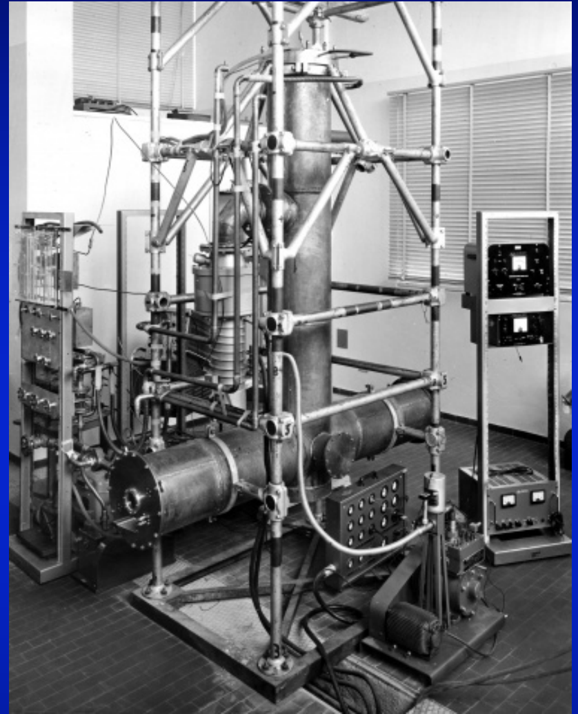
Bubble chamber during lab test
