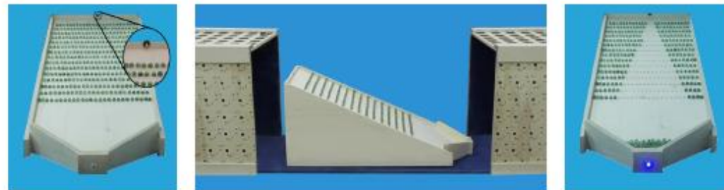
Figure 6. The model describing the avalanche process of electronic ionization taking place in the photomultiplier of a cosmic rays detector. One single glass marble descending along the inclined plane is not able to turn on the LED at the bottom, while the ball released by the electromagnet on the top (see the inset) can produce an avalanche that does turn on the LED.
