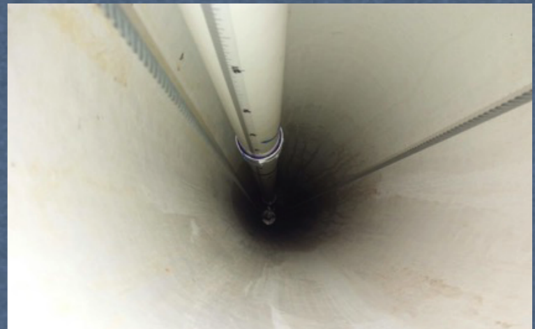
The BDX-Hodo lowered in well I
