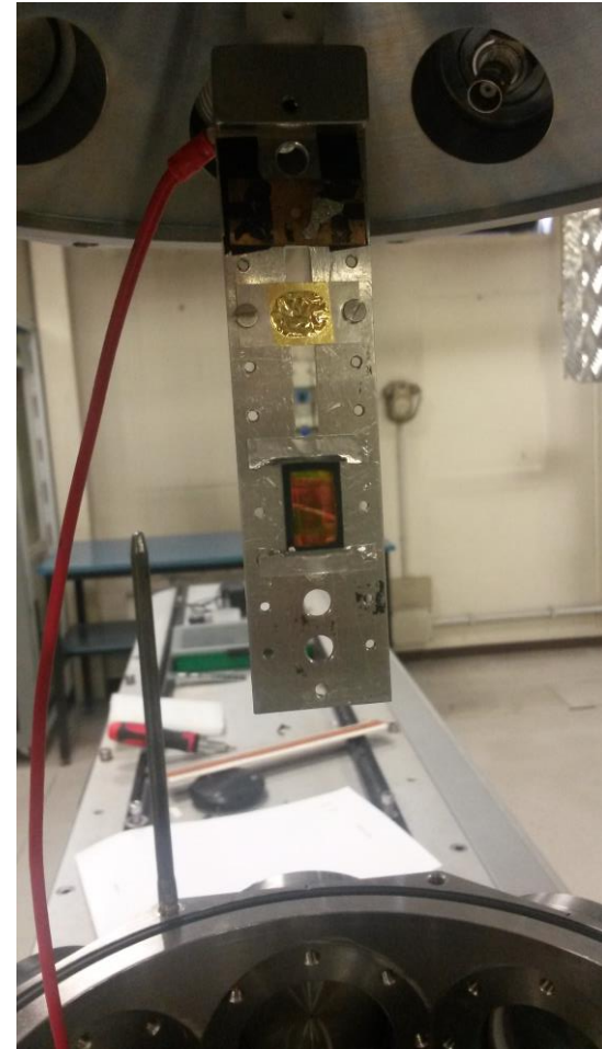
NAND Flash mounted on the sample holder inside the irradiation chamber at the AN2000 accelerator
