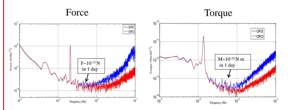
The cross-talk Force-Torque was experimentally tested to be lower than 0.1 % when the TM is centered.
