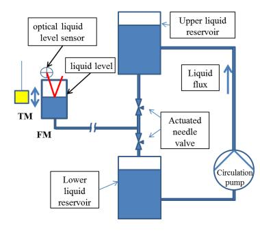
In a possible alternative scheme the FM is filled from an upper reservoir.
