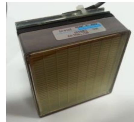
H12700 8x8 larger pixels Allows to reduce costs in the peripheral regions
