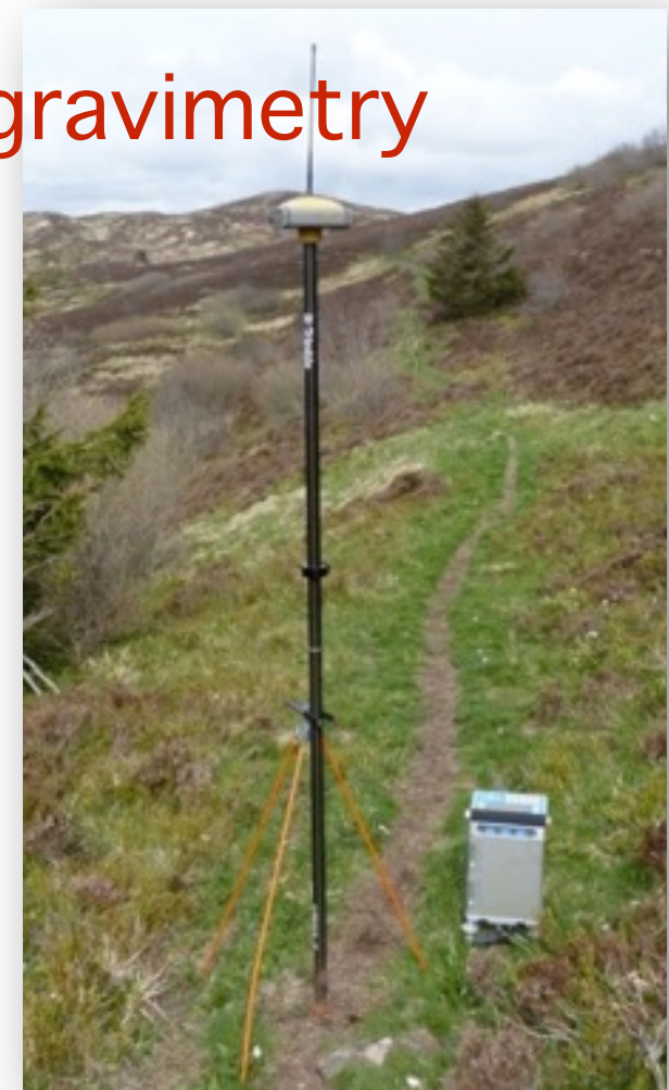
GPS and Scintrex CG5 gravimeter
