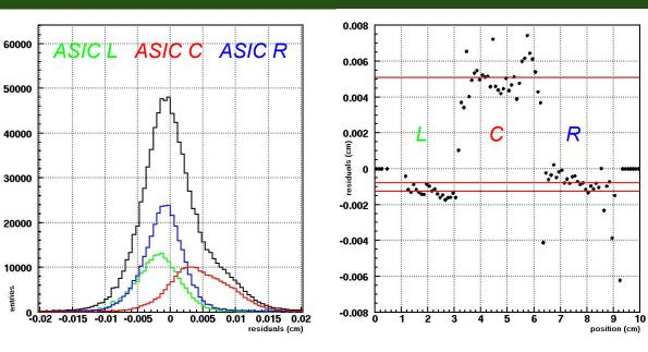
For the time being, a manual correction for the events passing through the central region of this layer should fix the problem...  $x(4,0) \rightarrow x(4,0) - 6.1E-3$  cm if  $x(4,0) \in (3.1,6.2)$  cm
