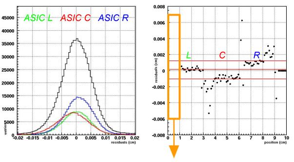
Leftmost centimeter absent in all y vista layers. This is due to a malfuntioning in 5y first 20 strips, which are dead → nonzero hits condition on 5y (which is required @ the moment of ASCII files creation) makes this pattern propagate to all the y vista layers
