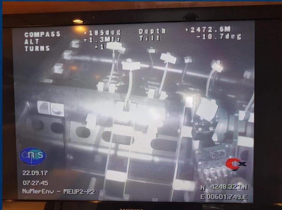
Wet-mateable connectors on the submarine node
