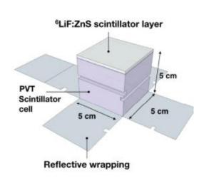
new segmented detector: optically isolated cubes readout by fibers
