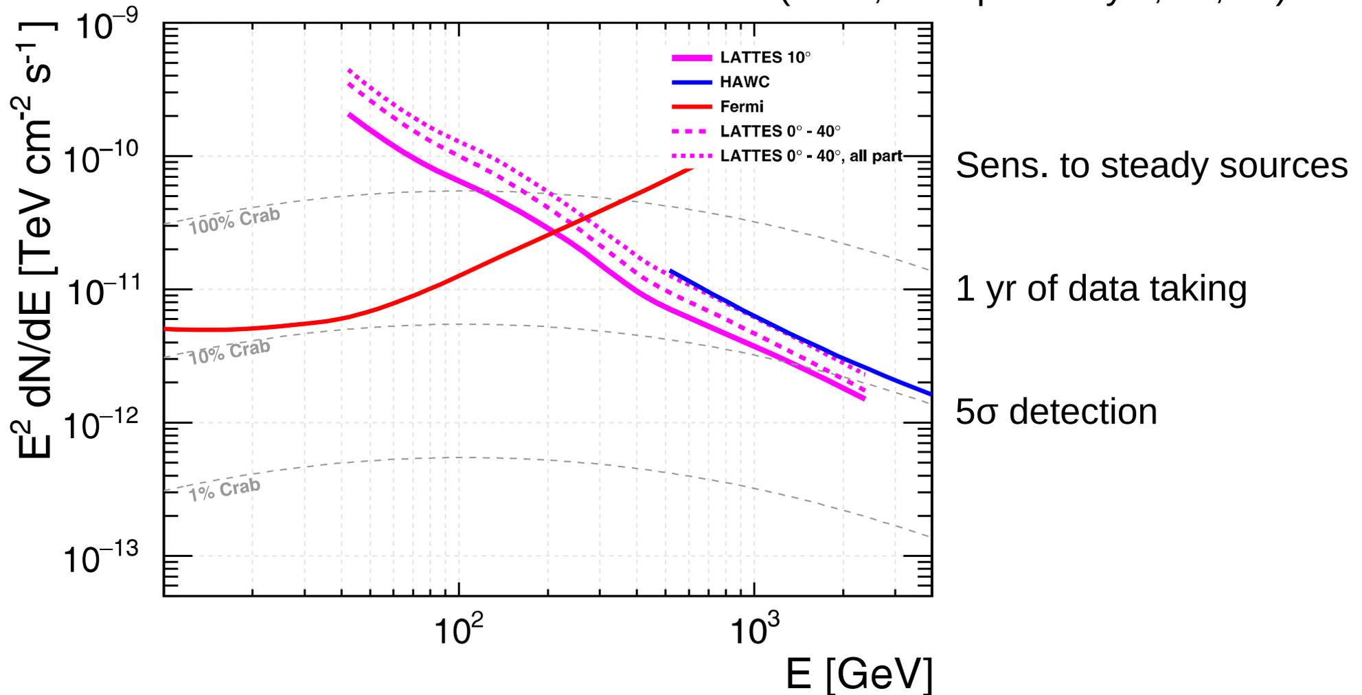
The LATTES concept design is estimated to extend the VHE monitoring capabilities down to 100 GeV, supporting pointed instruments like CTA.
