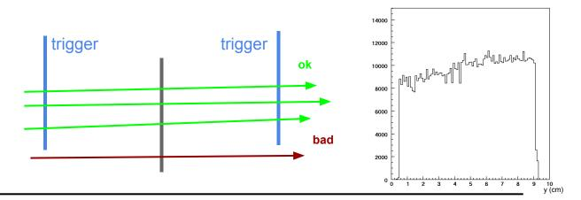
Layer 13y shows a particular structure in the right side (right to ~8cm). At first I thought it was a local inefficiency around ~8.2cm but then I noticed from alignment process results that this structure is present in upstream layers too (9y & 7y)  $\rightarrow$  this needs some investigation...
