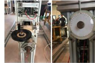
Figure 2: Left: the control knob of the telescope. Right: the angle meter.
