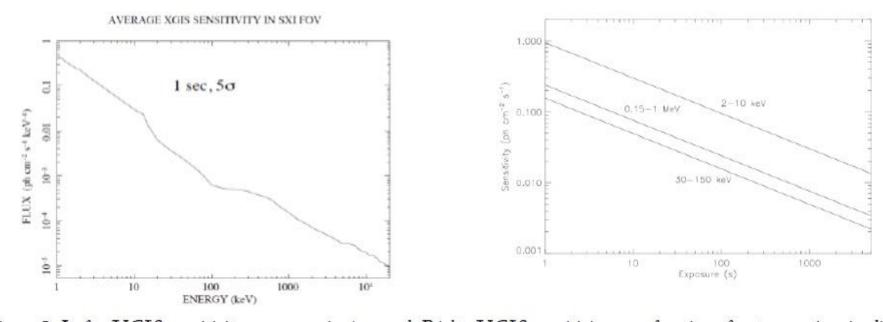
Figure 5: Left: XGIS sensitivity vs. energy in 1 second. Right: XGIS sensitivity as a function of exposure time in different bands.
