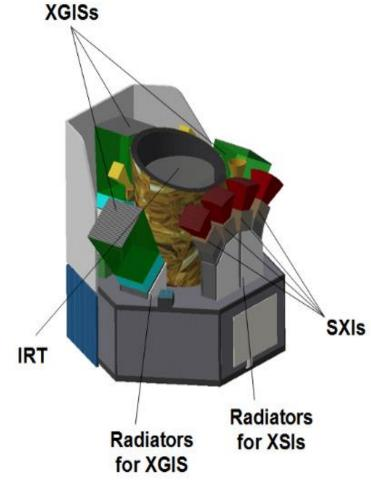
LEO (< 5°, ~600 km) Rapid slewing bus Prompt downlink ☐ THESEUS will have the ideal combination of instrumentation and mission profile for detecting all types of GRBs (long, short/hard, weak/soft, high-redshift), localizing them from a few arcmin down to arcsec and measure the redshift for a large fraction of them
