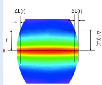
OPL distortions due to dependence of refractive index from temperature variation
