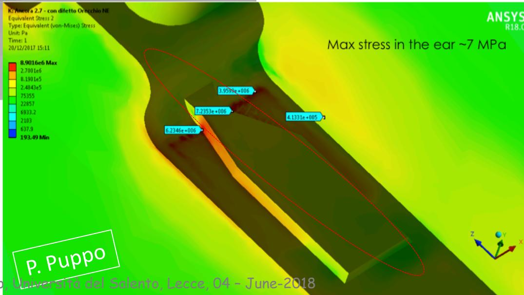
Thermal noise is OK if the ear holes are **not** filled with glue
