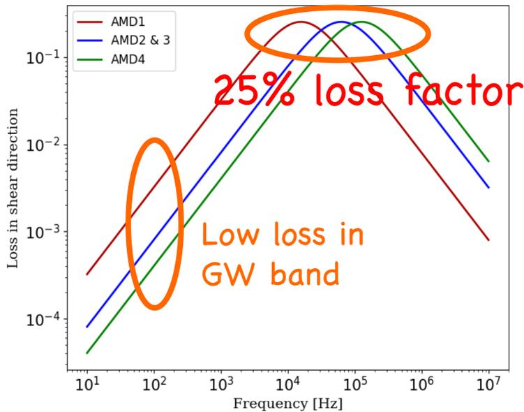
Pure mechanical damping mechanism developed by Virgo, under test using old V+ payload (Rome) and at EGO, through the dummy payload meant to check fused-silica suspension.
