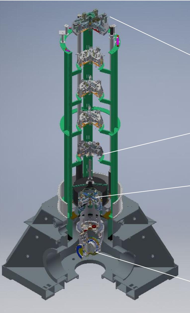
In AdV the first 5 stages of the Super-Attenuator (horizontal and vertical) are the same as in initial Virgo.
