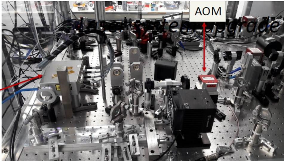
70 W amplifier replaced by a 100 W
