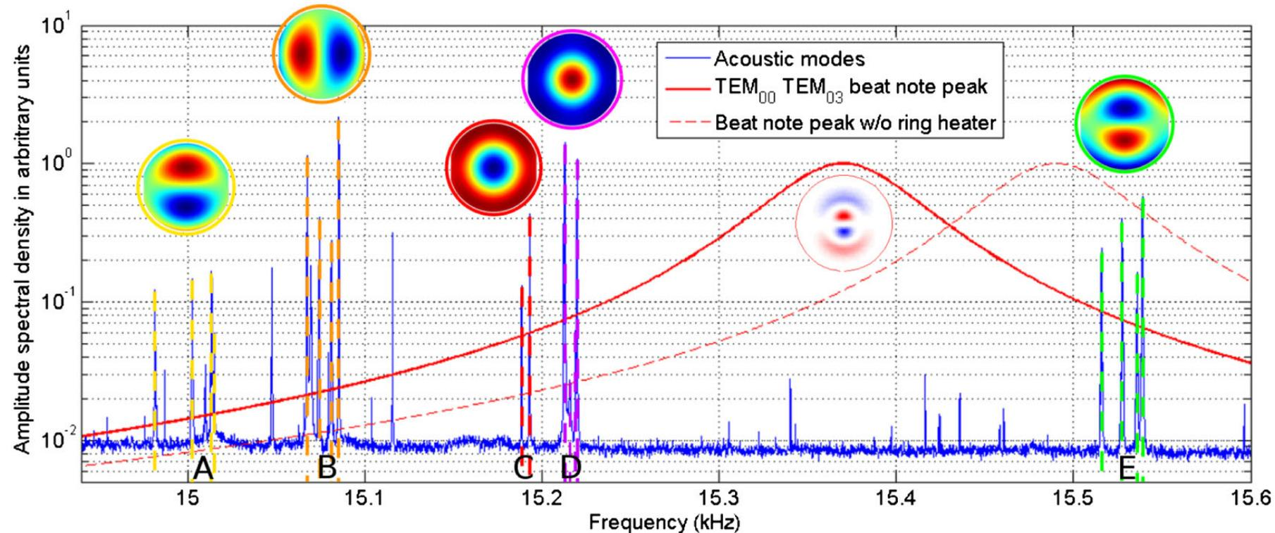
Thermal tuning with the RH changes the Mirror radius of curvature and shifts the beating note far from the most critical mode (E)
