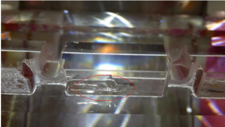
Mechanical stress in the damaged ear, after gluing of anchors, is far from breaking strength
