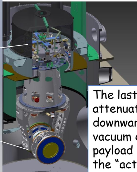
The last filter of the Super attenuator, prolonged downwards, is in the same vacuum environment of the payload and surrounds it: the "actuation cage".
