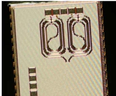
Optical modulation is obtained in silicon photonics circuits via electro-optical effect (plasma dispersion).
