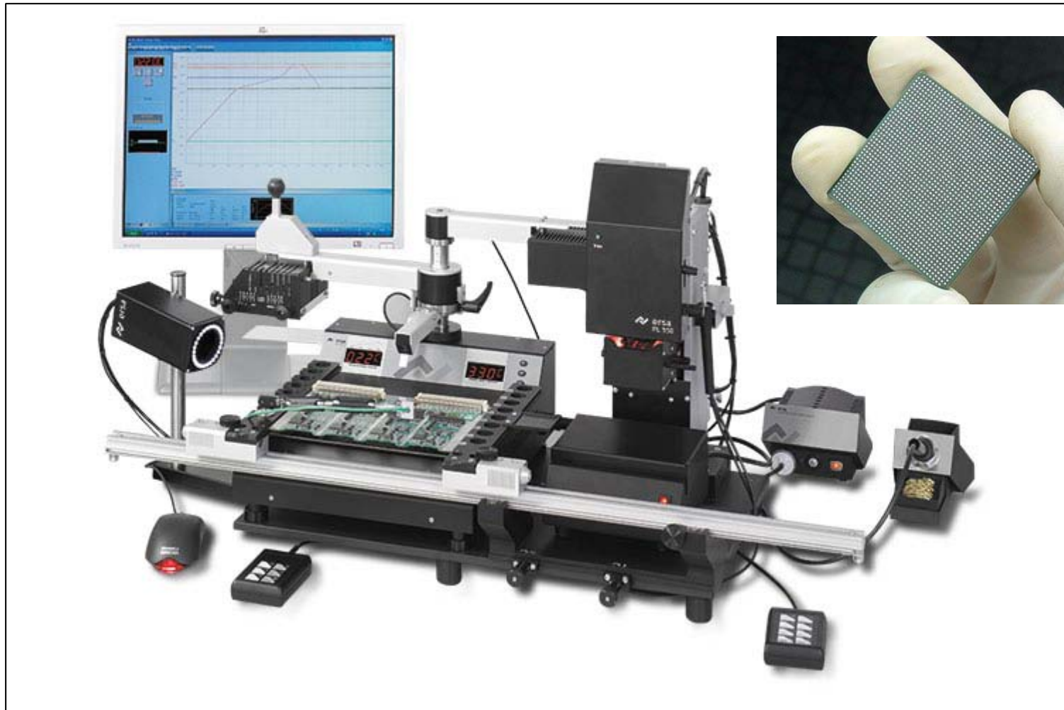
SMT- BGA rework machine and prototypes assembly
