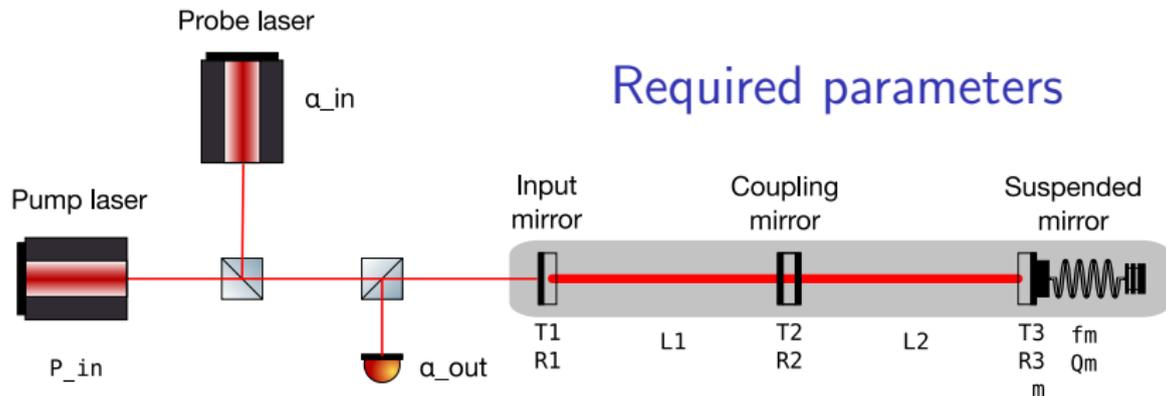
Resolved sideband damping in a coupled cavity system.
