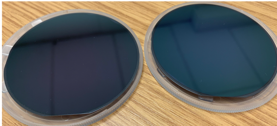
300nm GaP coatings on Si
