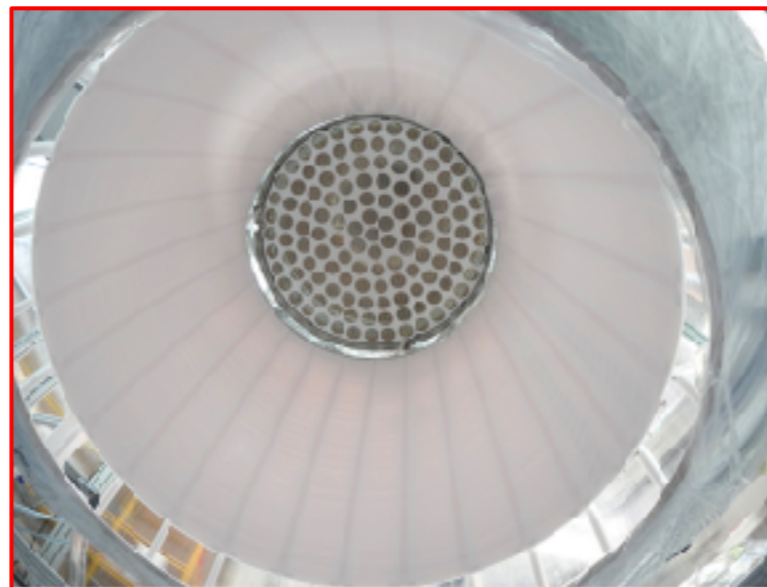
127 PMTs in the top array
