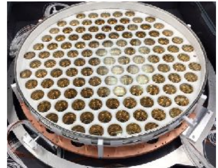
121 PMTs in the bottom array
