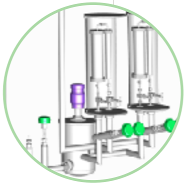
LXe Purification To achieve fast cleaning of the large LXe volume (5000 SLPM)
