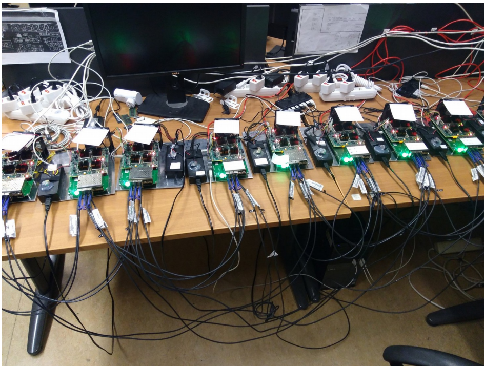
ExaNeST 8-nodes prototype (as of 18/5/18) with INFN ExaNet interconnect
