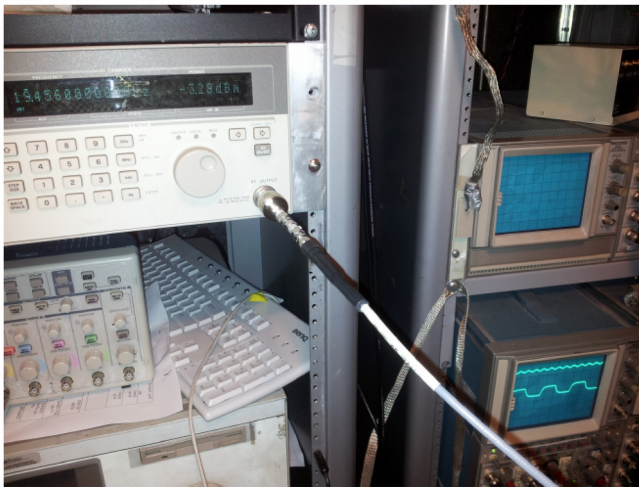
Figura 5. Setup logica ERSFQ, Freq. In =19,456 GHz, Freq. Out = 2375 KHz. Freq. ref.=593,75KHz.
