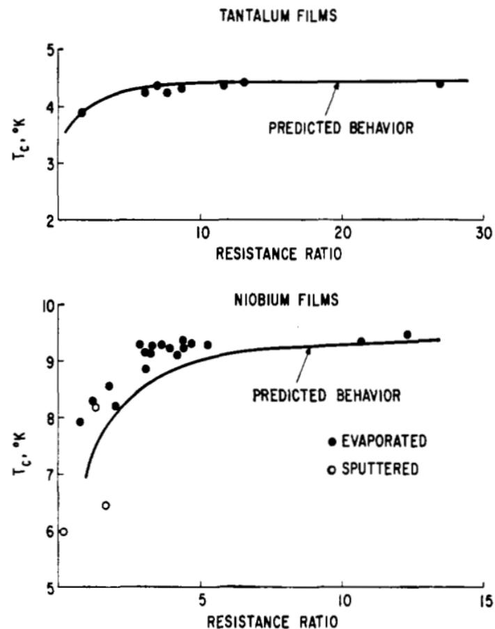
Fig. 3—Critical temperatures of Niobium and Tantalum films as a function of their resistance ratio.
