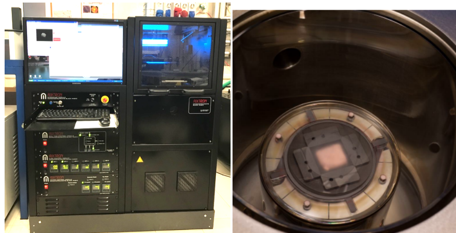
Aixtron Black-Magic: Cold-wall reactor enabling very fast graphene synthesis on cm-scale sample
